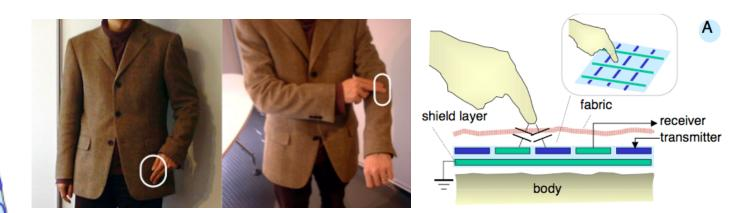
Advances in fabric manufacturing and electronics allow for clothes to be used for networking, and for gesture detection.
