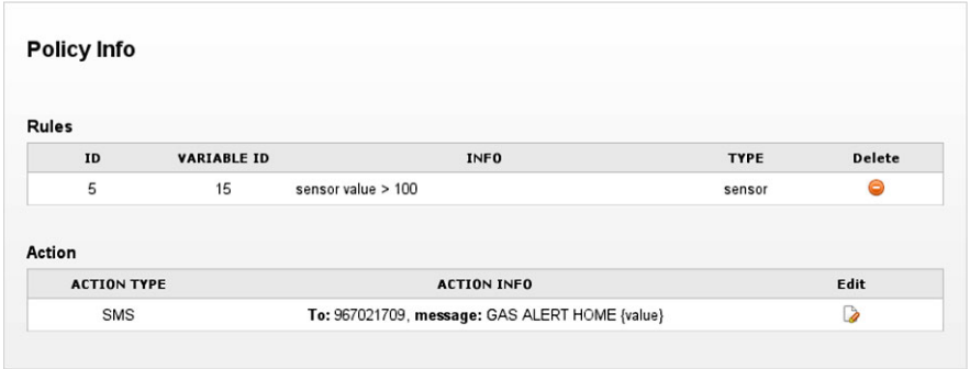
Fig. 7.6 A policy to alert via SMS when there is a gas leak (gas_value > 100)
