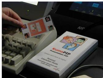
Figure 4. A user logs into an embedded PIP interface by swiping an RFID card.
