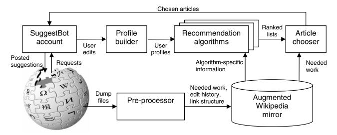
Figure 3: SuggestBot's architecture. It pre-processes Wikipedia data, combining it with user profiles based on edit history as input to several recommendation engines. It combines the results of the engines in order to make suggestions.
